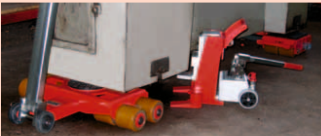
Castors with ball bearings guarantee easy movement
