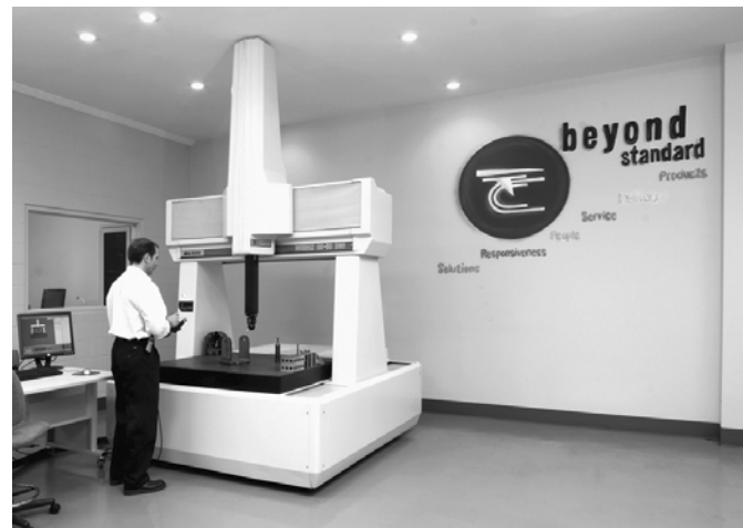
A 1200 x 1000 x 800mm Sheffield Coordinate Measuring Machine is used to inspect parts and assemblies for precision fit.
