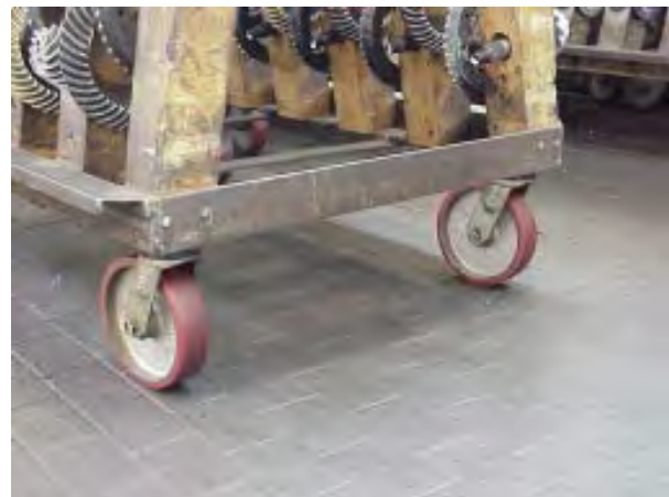
Spindle rack for gear blanks. T/R compound soft polyurethane is floor protective and will not pick up machine shavings or debris.
