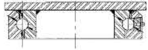
SWIVEL CROSS SECTION
